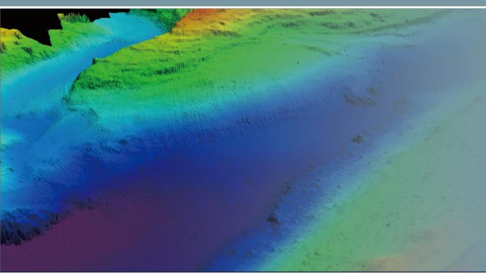
MS8240 is born to cater complex underwater terrain changes and can obtain clean and high-resolution data quality. This multibeam sonar can output 150~450khz continuous frequency conversion and also supports 700khz ultra-high frequency signal output, which can capture ultra-high resolution 3D topographic data and present excellent details for your survey work.
