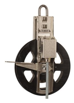
The pulley is opened to allow the cable to be fitted or removed by releasing the axle clip, then depressing the axle lever and swinging up the arm on which the axle clip is fitted.
