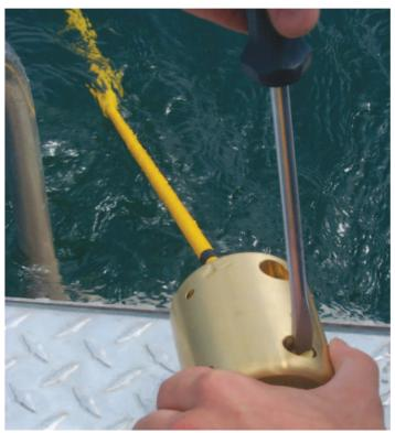
Brass tow cable weight attached to MMC's cable
